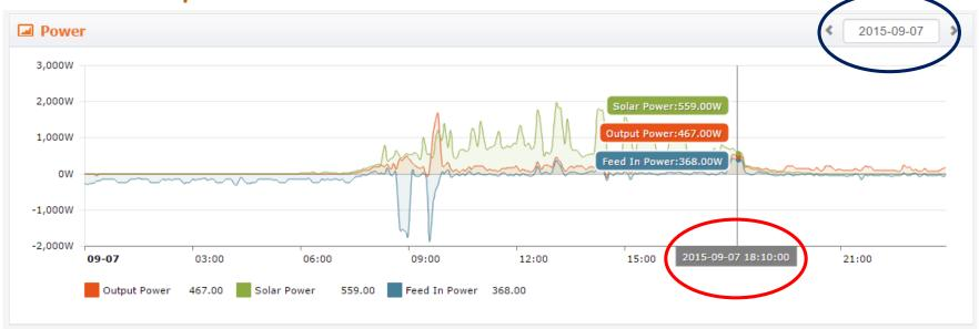
This is the main graph you will use, as you can see there are three main entities; Solar Power, Output Power and Feed In Power. All are measured in watts (W). The grey line represents what time of day you are looking at, as you can see in the image above we are looking at what is happening at 18:10:00 or 6.10pm (circled in red) on the 07/09/15 (circled in blue). You can select a date by simply clicking the arrows either side of the date to choose another date.
