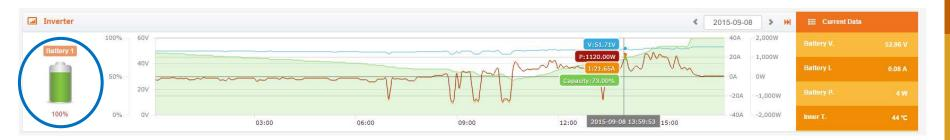
The battery image on the left (please note the 'Battery 1' is all of your batteries combined) gives you a clear indication of the amount of charge inside your battery, as you can see on this image (circled in blue), the battery is at 100%. \*Please note that the battery image is a real time reading so it will not correspond with the part of the graph I have highlighted.
